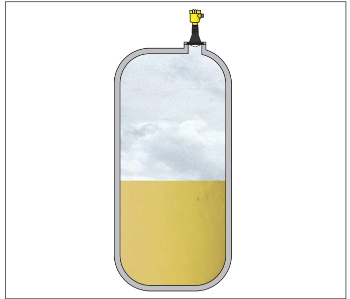
Fig. 26: Level measurement in an acid tank with VEGAPULS 61
